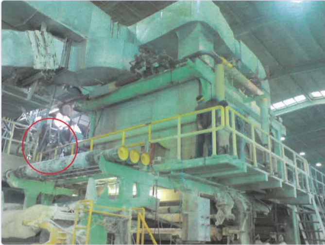
The Yankee dryer; the Jetomat is circled
